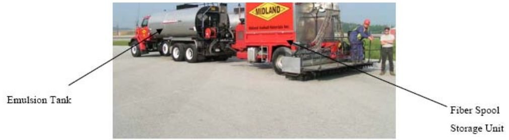
Figure 2: Truck with an emulsion tank and Fiber Storage Unit
