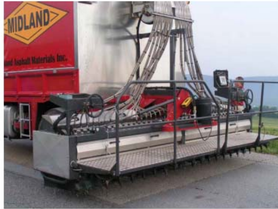
Figure 3: Rows of nozzles spraying the emulsion and fibers
